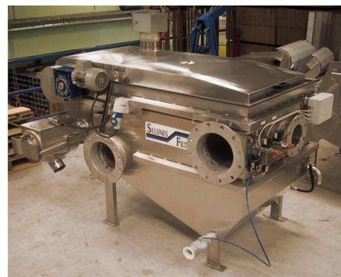
Salsnes filter does not require to use of additional chemicals, such as coagulants and flocculants. Power consumption for treatment wastewater and sludge dewatering is at the level  $0,06 \text{ kWh/m}^3$ . To clean filter mesh is used compressed air from the blower, which is the part of the filter, and in the case of plants with a high fat content, the mesh is washed by hot water several time a day (about 20 liters per wash).
